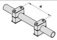
The recommended distances between clamps stated below are standard values and are valid for static loads.
