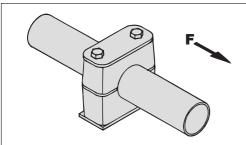
All tightening torques and maximum loads in pipe direction refer to clamps with cover plates and hexagon head bolts acc. to DIN EN ISO 4014/4017 (DIN 931/933).
