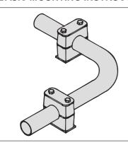
Pipe bends should be supported by STAUFF clamps as near to the bends as possible.
