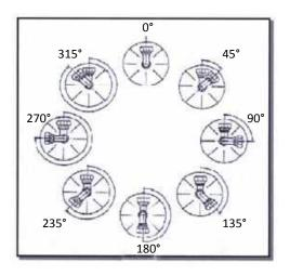
Refer to the following picture to define the correct fitting orientation.
