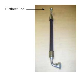
Keep straight the further end and rotate <u>clockwise</u> the closest end of the requested angle.
