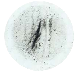
Residual particles from a hydraulic hose, not cleaned
