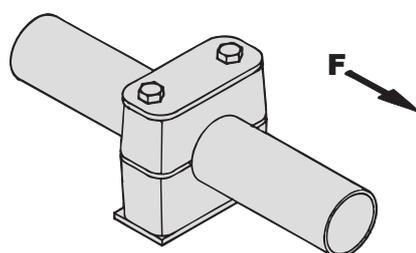
All tightening torques and maximum loads in pipe direction refer to clamps with cover plates and hexagon head bolts acc. to DIN EN ISO 4014/4017 (DIN 931/933).
