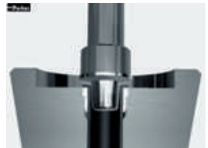
The front surface is continuously rolled and compressed. From the inside, the tube surface is slightly expanded to clamp the sleeve
