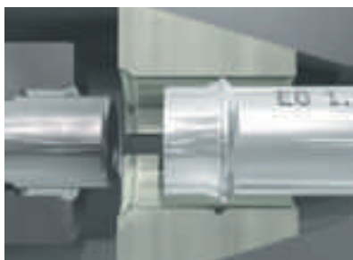
The tube end is released and ready for attaching the EO-2 seal
