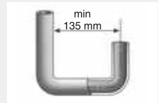
● Minimum clearance of U-shape bends
