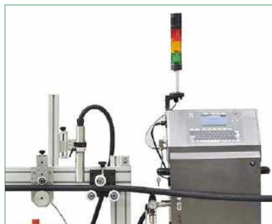
▲ MARCATRICE CON CONTROLLO ENCODER MARKING DEVICE WITH ENCODER CONTROL
