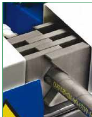
◀ MORSA PNEUMATICA AUTO-CENTRANTE - SELF-CENTERING PNEUMATIC VICE
